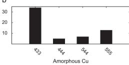
**Fig. 9.** (a) Calculated histogram for Zr–Zr pair coordination number. The most abundant pairs are 555 and 544, indicating the dominance of perfect icosahedral order and other different type of distorted icosahedral order, respectively. (b) Calculated histogram for Cu–Cu pair coordination number. The most abundant pairs are 433 and 555, indicating the dominance of a type of distorted icosahedral order.
