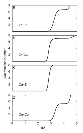
**Fig. 2.** Calculated coordination number (CN) for  $Cu_{46}Zr_{54}$  crystalline phase. (a) Zr-Zr (CN=7), (b) Zr-Cu (CN=7), (c) Cu-Zr (CN=8), and (d) Cu-Cu (CN=5).
