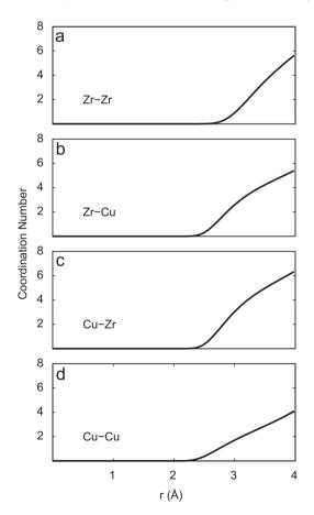
Fig. 5. (a)–(d) Calculated coordination number for  $\text{Cu}_{46}\text{Zr}_{54}$  liquid phase.
