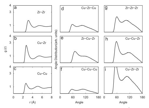
**Fig. 4.** (a)–(c) Calculated pair-correlation function for  $Cu_{46}Zr_{54}$  crystalline phase: two main peaks are located at (a) 3.1 and 5.5 Å for Zr–Zr, (b) 2.7 and 5.2 Å for Cu–Zr, finally (c) 2.6 and 5 Å for Cu–Cu (c). (d)–(i) Calculated angular distribution for the crystalline phase: the main peaks are located at (d) 58° and 114° for Cu–Zr–Cu, (e) 70° and 110° for Zr–Cu–Zr, (f) 58° and 110° for Cu–Cu–Cu and (g) Zr–Zr–Zr. Finally, (h) 58° and 110° for Cu–Cu–Zr bond angles.
