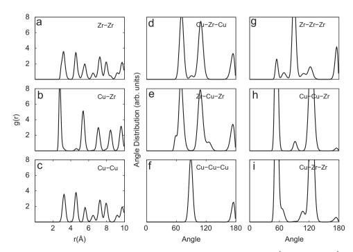
**Fig. 1.** (a)–(c) Calculated pair-correlation function for  $Cu_{46}Zr_{54}$  crystalline phase: the main peaks are located at (a) 3.18 Å for Zr–Zr, (b) 2.76 Å for Cu–Zr and (c) 3.22 Å for Cu–Cu. (d)–(i) Calculated angular distribution for the crystalline phase: the main peaks are located at (d) 70° and 110° for Cu–Zr–Cu and (e) Zr–Cu–Zr, (f) 90° and 175° for Cu–Cu–Cu and (g) Zr–Zr–Zr. Finally, (h) 54° and 125° for Cu–Cu–Zr and (i) Cu–Zr–Zr bond angles.
