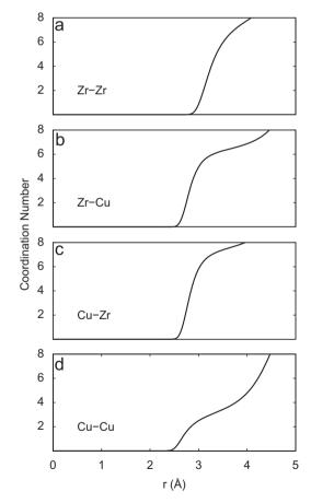
**Fig. 8.** (a)–(d) Calculated coordination number for Cu<sub>46</sub>Zr<sub>54</sub> amorphous phase.
