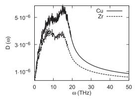
**Fig. 10.** Calculated vibrational density of states for  $Cu_{46}Zr_{54}$  amorphous phase. Solid line represents the partial vibrational density of states for Cu and the dashed line is the partial vibrational density states for Zr.
