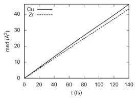
**Fig. 6.** Calculated diffusion coefficient for  $Cu_{46}Zr_{54}$  liquid phase. The diffusion coefficient for Cu (solid line) is 0.061 Å $^2$  fs $^{-1}$  and for Zr (dashed line) is 0.051 Å $^2$  fs $^{-1}$ .
