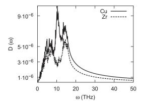
**Fig. 3.** Calculated vibrational density of states for  $Cu_{46}Zr_{54}$  crystalline phase. Solid line represents the partial vibrational density of states for Cu and the dashed line is the partial vibrational density states for Zr.
